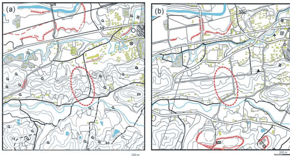
Fig. 4a,b Contour maps of the Tsukidate area in 1962 (a) and 2001 (b), respectively. The Tsukidate landslide was triggered within the red circle in May 2003
