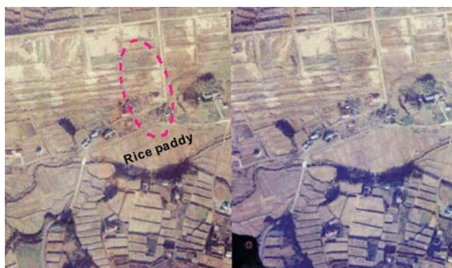
Fig. 5 Stereo-pair air photographs of the Tsukidate landslide site before the earthquake, taken by the Geographical Survey Institute of Ministry of Land, Infrastructure and Transportation. Source area of the Tsukidate landslide is located inside the red circle
